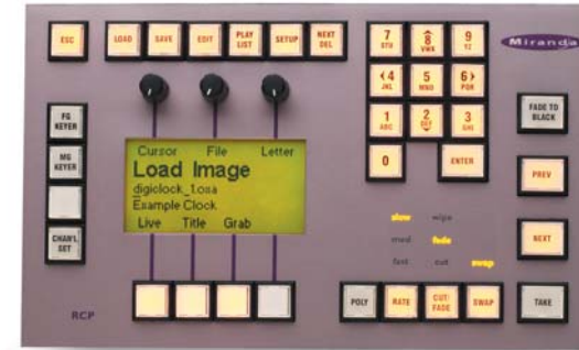
Oxtel-RCP remote control panel
